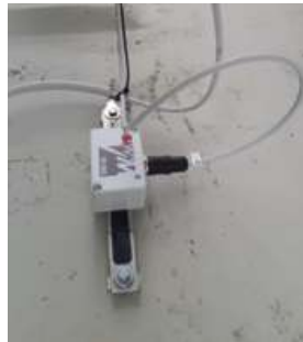
Installation of the SiWIM sensors under the bridge.
