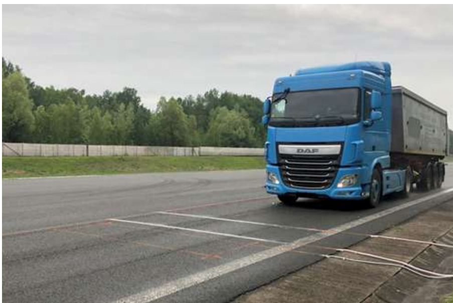
Kistler WIM system during high speed tests.
