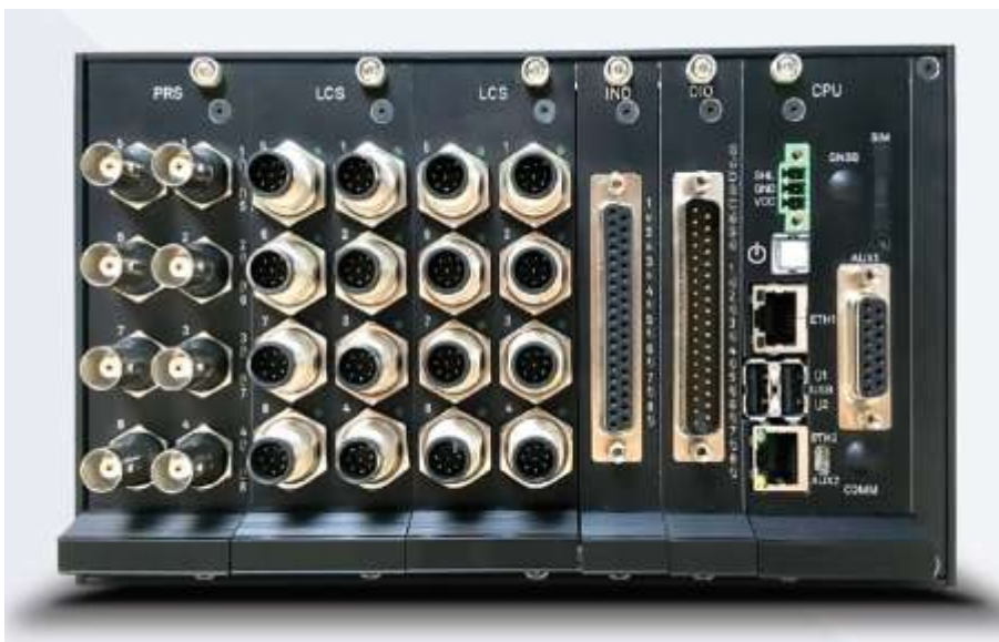
CAMEA WIM system electronics.
