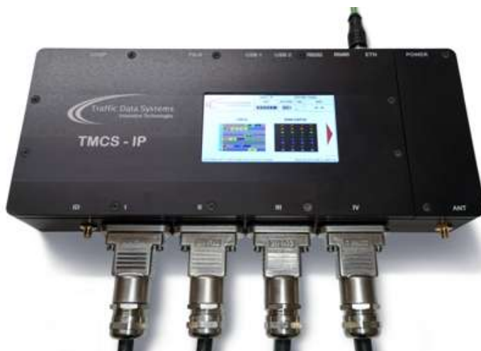
TMCS-IP with integral WIM-DSP32
