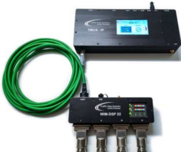
TMCS-IP without integral WIM-DSP32
