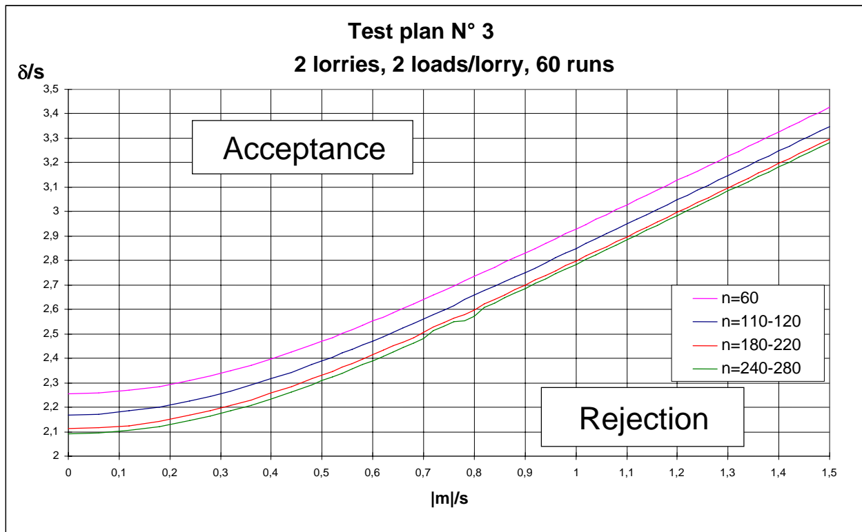
Figure A-2-2 - Chart of acceptance (Test plan N° 3, level of confidence 95%)
