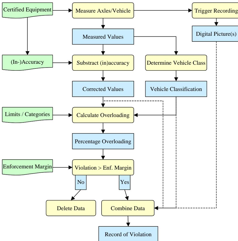
**Figure 3.3, Procedure for automatic enforcement.**
