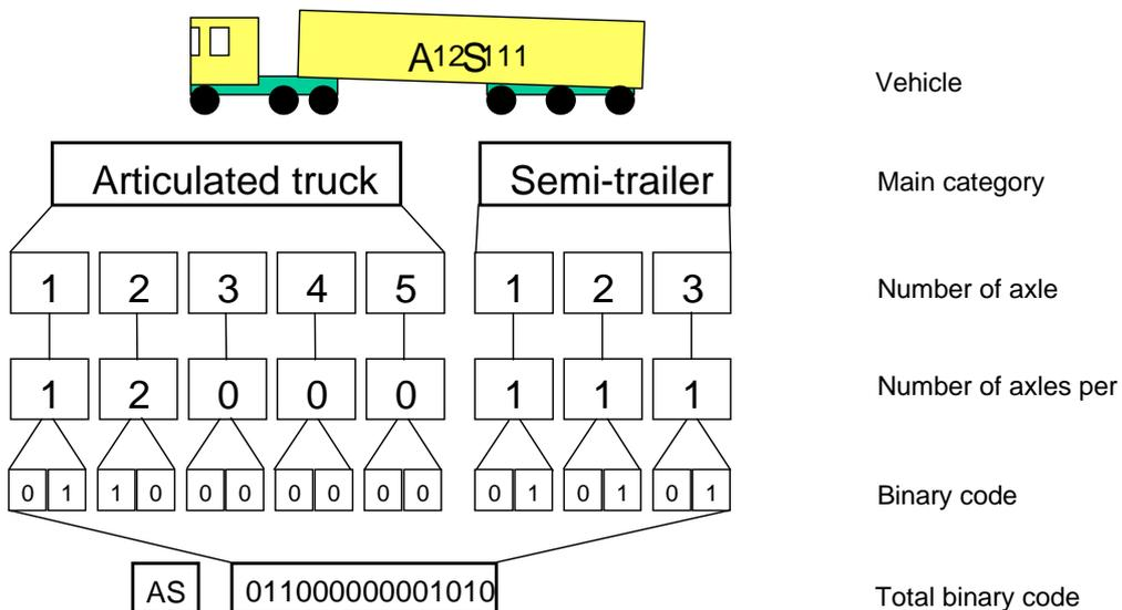
**Figure 3.4. Determination of the total binary code for A12S111**
