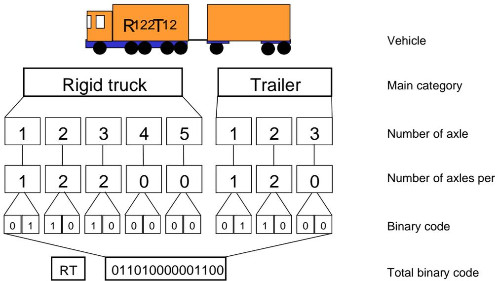
**Figure 3.5, determination of the total binary code for R122T12**
