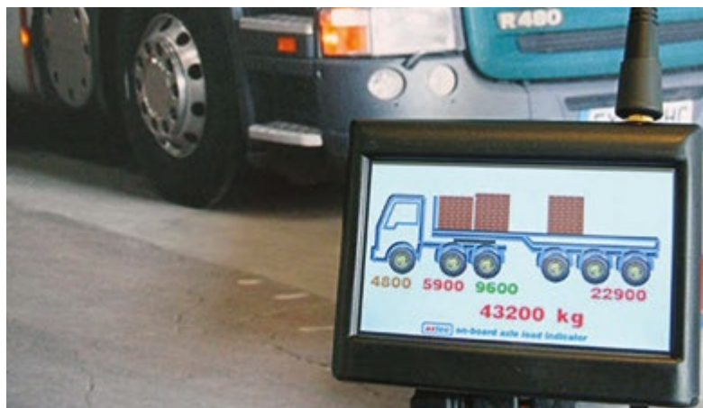
Figure 3.8: Display of On-Board Weighing measurements
