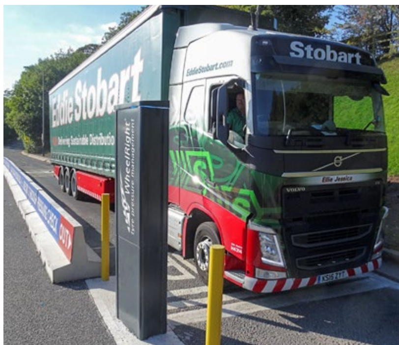
Figure 4.4: WIM system used for tyre management
