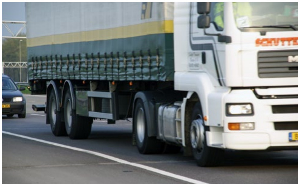
Figure 6.1: A 4-axle calibration truck passing WIM sensors
